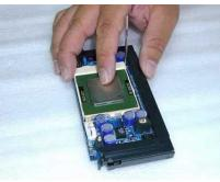
Installing the processor in the PL-P3/SMP. (1)
